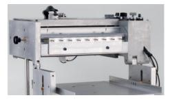
To optimize the usage of products with different textures, **two series of nozzles** with 2 and 5 mm diameter are provided.
