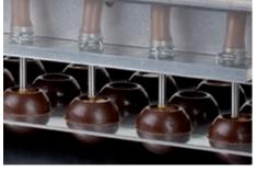
The amount of filling product to be dosed and the filling rate can be easily controlled by tuning the tank pressure (0-1 bar) and the opening time.
